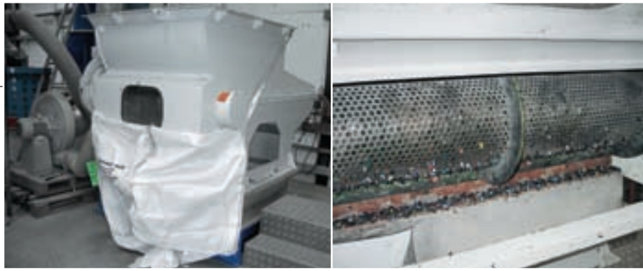
Fig. 1 Shredder for the crushing of the capacitors (type: Vecoplan VAZ 105/120, 18.5 kW, approx. 550 kg/h) and 8 mm sieve used for IT/CE < 1 cm (sample N° 7)
