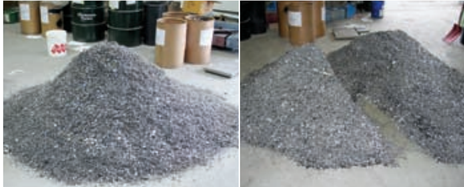
Fig. 2 Splitting and reduction of samples by means of „coning and quartering“ of the shredded material
